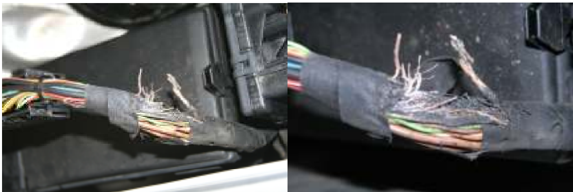
Main wiring to traction control ECU
