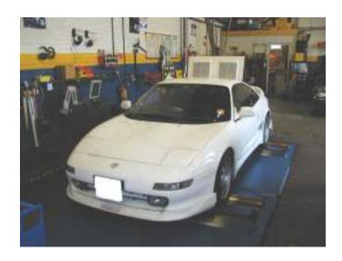
WE WERE ASKED TO DIAGNOSE A PROBLEM WITH A TOYOTA MR2 TURBO. THE HISTORY WITH THE VEHICLE WAS THAT IT HAD DEVELOPED A MISFIRE UNDER LOAD AFTER BEING FILLED WITH DIESEL.
